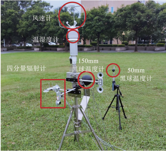
图2 现场观测仪器装置 Fig.2 Instruments for field observation
