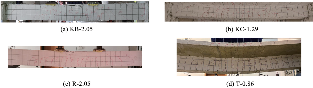
图 7 试验梁破坏形态 Fig. 7 Failure mode of beam specimens
