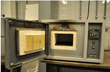
图 1 可控温电热炉 Fig.1 Temperature-controllable furnace
