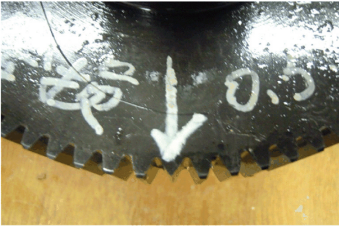
图 3 齿轮磨损 50%示意 Fig.3 Wear of gear of 50%
