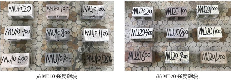
图 6 两个强度砌块历经各温度后的形态 Fig. 6 Appearance morphology of blocks for two strength grades after exposure to different temperatures
