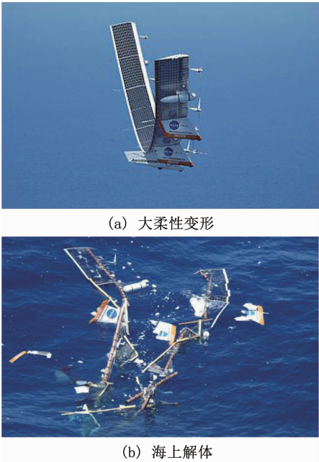
图 8 “太阳神”无人机非线性气动弹性问题 Fig. 8 Nonlinear aeroelastic of the “Helios” UAV
