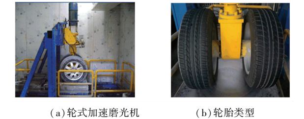
图 1 温控轮式加速磨光系统 Fig.1 Thermo-control and accelerated wheel tracking polishing system
