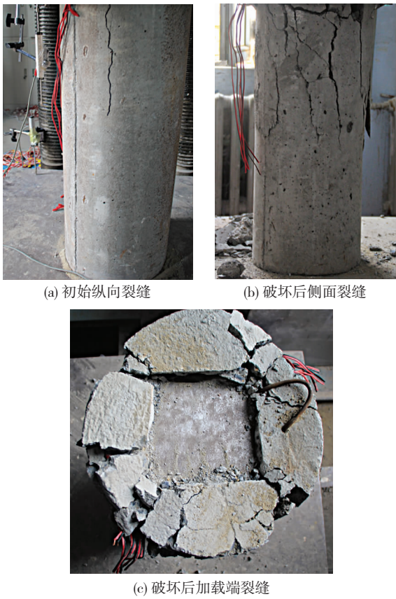
图 4 配置螺旋式间接钢筋的混凝土试件裂缝分布 Fig. 4 Distribution of cracks in concrete specimens with spiral indirect steel bars
