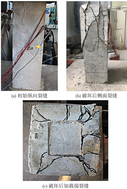
图 5 配置网格式间接钢筋的混凝土试件裂缝分布 Fig. 5 Distribution of cracks in concrete specimens with meshed indirect steel bars
