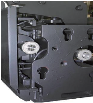
图 4 熨平板结构 Fig.4 Structure of screed
